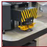
6mm Thickness Maximum Ø14mm Punching capacity
