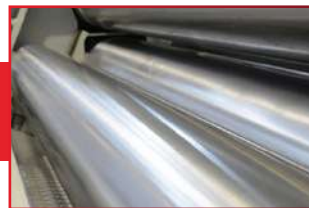
Induction hardened, polished rolls
