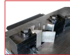
V-Pressbrake Punch & Die included as standard
