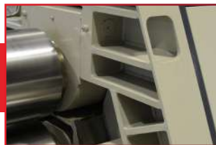
Welded rigid frames
